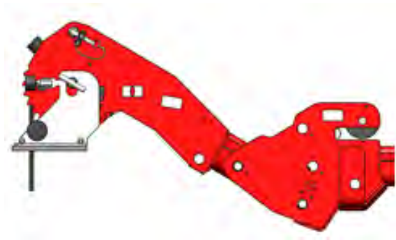
Figuur 4.10 Adjustable section upper limit
