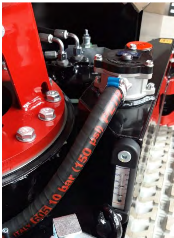
Figuur 4.1 Checking oil level
