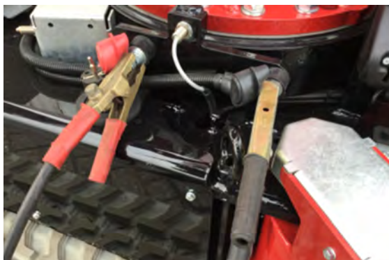
Figuur 5.5 Emergency charging points
