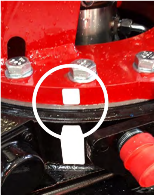
Figuur 7.2 Centre position of crane column
