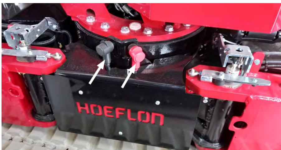
Figure 5.6 Bornes de recharge de secours
