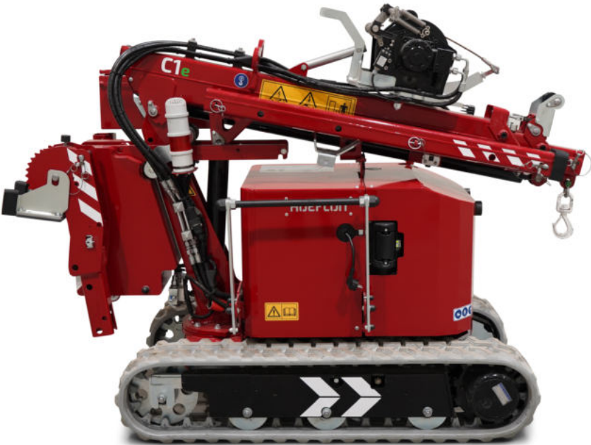
Figure 7.1 Crane in transport position
