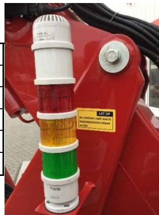
Figure 7 : colonne de signal
